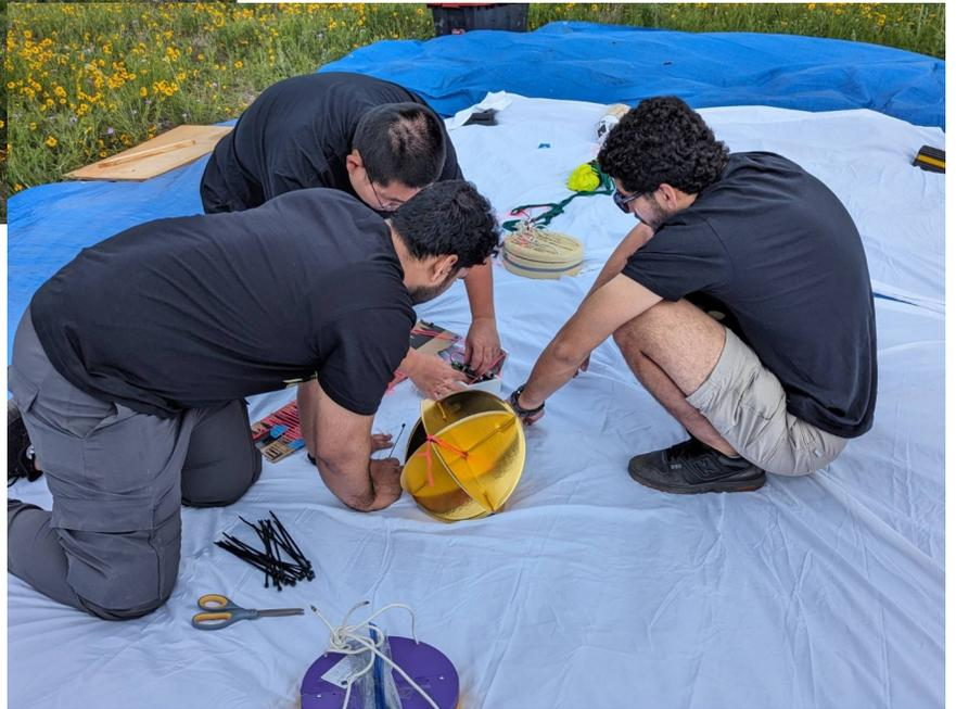
Attaching the radar reflector
